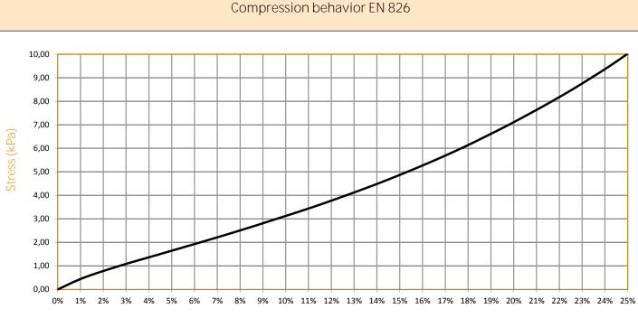
Note: maximum deflection (%) assessed on 1 sqm with a rubber insert equal to 5% of the surface.
