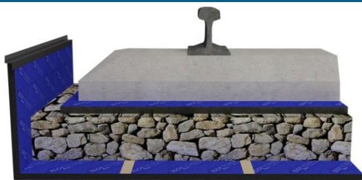
Over ballast sleeper pads
